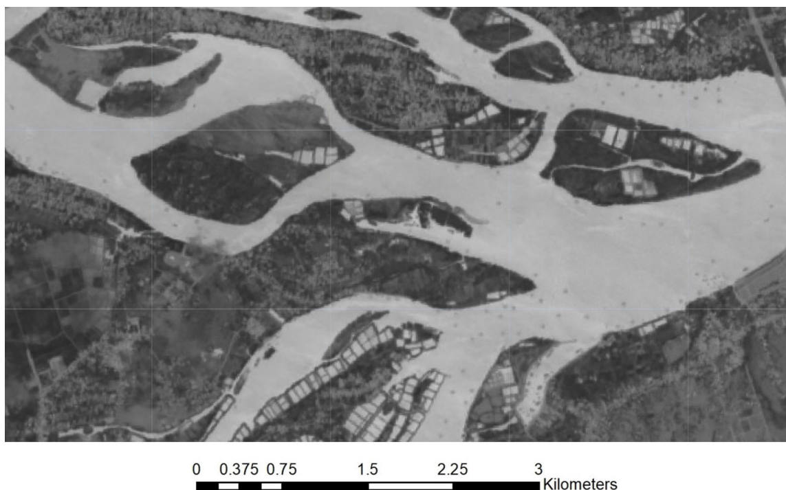
Fig. 13. NDWI index in the test area 1, calculated from Sentinel 2A image, June 11, 2020
